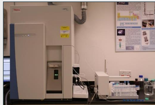
感應耦合電漿質譜分析儀 Thermo iCAP Qs Inductively Coupled Plasma Mass Spectrometer
