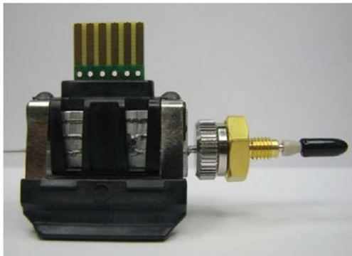
Pictured Above: Active Pre-Heater prior to modifications made for "Plus" Instruments
